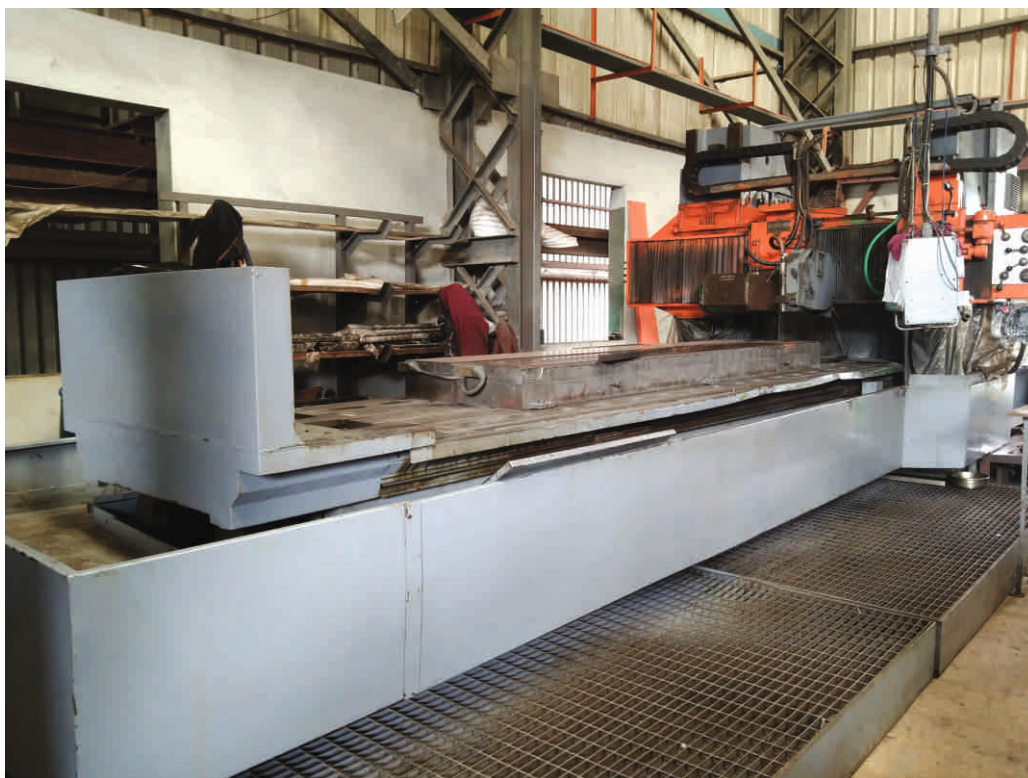
Figure 2 . Italian Sideway Grinding Machine Accuracy within 5 microns
